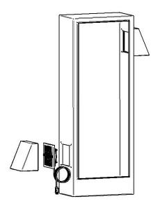
In this image, a standard installation shows where the dirt and particulate will enter the enclosure and be pulled in by the fans on your drives and devices. Filters or not, contamination is invited in by this *open loop* approach.
